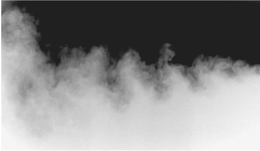
Figure 2: View of a spatially developing Rayleigh-Taylor instability from experiments by Banerjee, Kraft, and Andrews [BKA10, p. 133] for A = 0.47 . The white fluid is lighter than the dark fluid. The fluids are moving to the left at 1.65 m/s.
